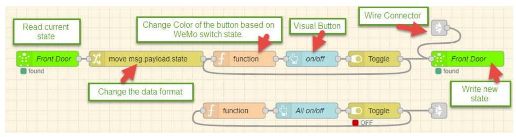
This is a portion of a flow that controls Belkin WeMo switches. The blue color nodes display a button in the Dashboard.
