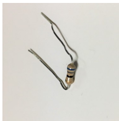
Leads Bent (Step c)
