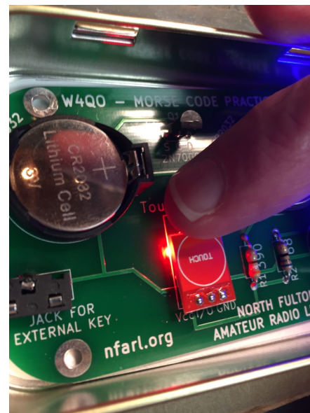
When “Keyed” the LED on the bottom of the Touch Module illuminates
