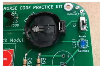
BAT1 soldered in place
