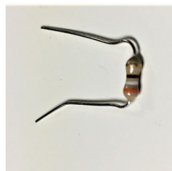
Leads Bent (Step “c”)
