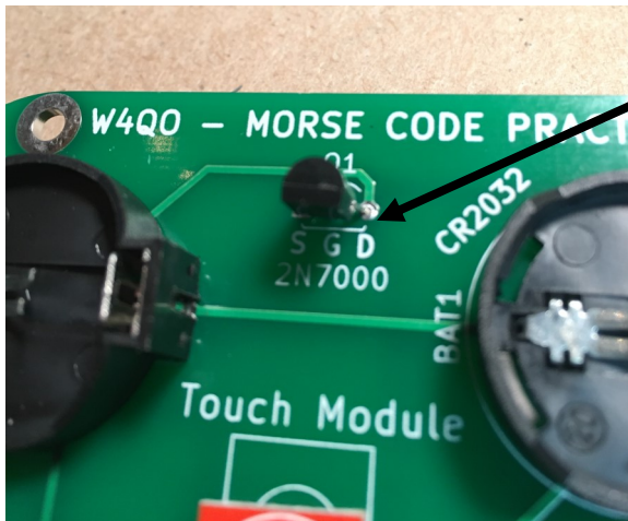
Q1 Soldered in place
