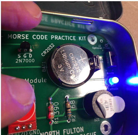
When “Keyed” the LED1 illuminates
