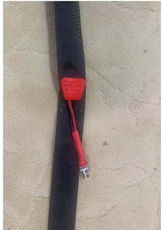
Right: the back side of the fabric, showing the feedline pigtail assembly fastened to the antenna. The 3D printed red mounting plate is bolted to the pigtail and the fabric/tape assembly. Note the BNC connector.
