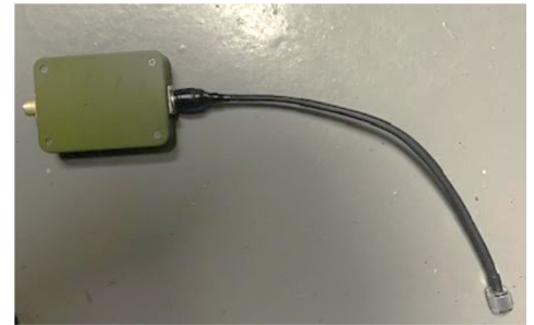
Figure #6 Feedpoint Choke
