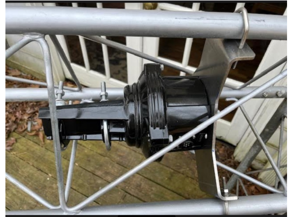
Figure #4 – Rotor assembly installed
