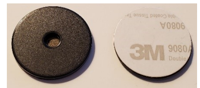
NFC tag used on metal surfaces. Notice the black substrate backing.
