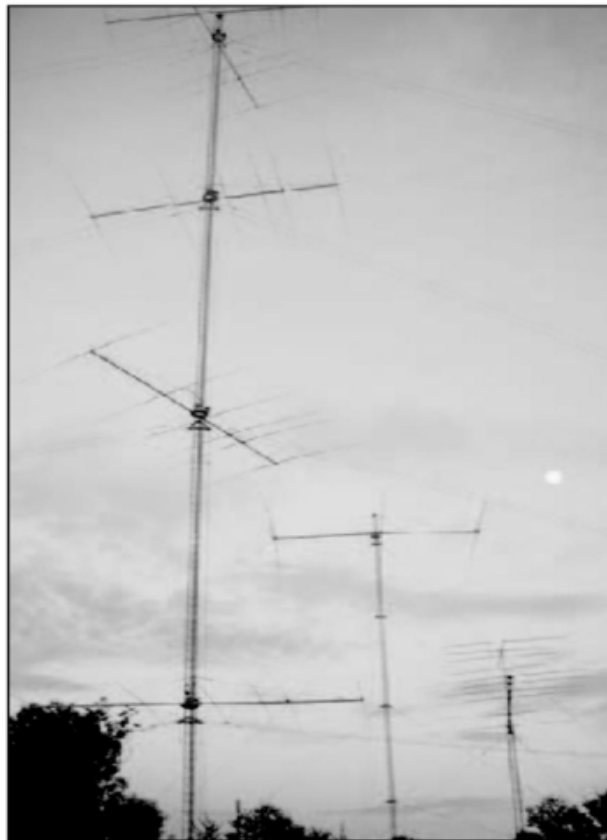
Figure 1 — The moon sets over four stacked 20 meter beams and a 3 element 80 meter beam — and this is only part of the NR5M antenna farm.
