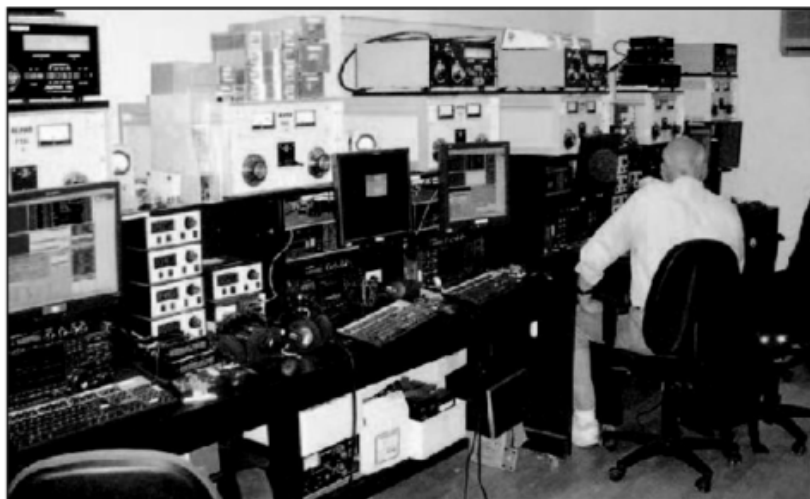
Figure 2 — The war room at NR5M. Two of the single-band stations. Each includes a separate transceiver and amplifier for running and sweeping. All stations are networked to share log information. This is the nerve center and front line for the NR5M team's radiosport action.
