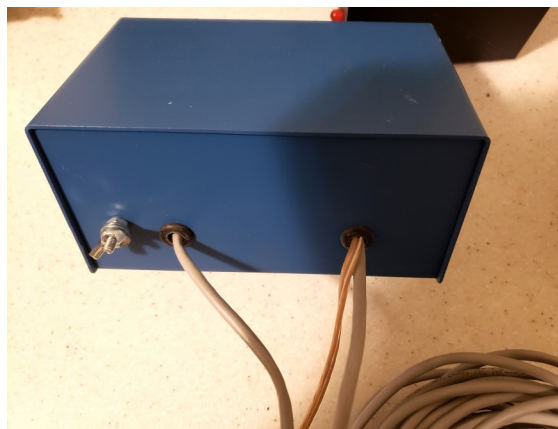
Figure 4—Ground stud added to control case
