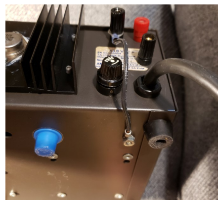
Figure 2– Added grounding wire
