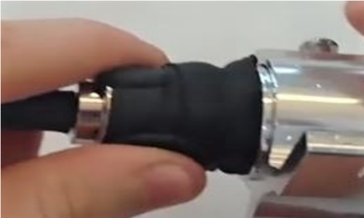
Figure 4. A screen grab from YouTube demonstrating one and possibly two mistakes. A conforming putty-like material is used to “seal” the front of a PL-259 connector shell to a grounding block while leaving the back of the connector wide open to water ingress. Also, the product description makes no mention of the material’s UV tolerance. Will it last in the sun? The manufacturer makes no claim.
