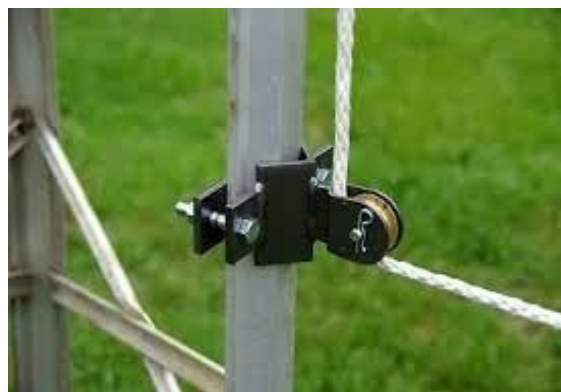
Figure 3. An eBay sourced 90 degree pulley sold without specifications of any kind. To be avoided!
