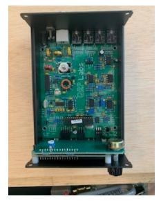
**QRP Labs 50 Watt Amplifier:** This is used with the QRP Labs Transceiver. It is a little more difficult to wind the coils on this unit. This work is a test of patience. A very good kit and fun
