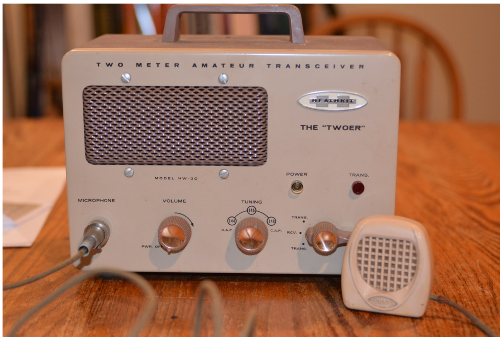
Superregenerative detector with RF amplifier, about 5 watts input, crystal controlled. Also known as a "Benton Harbor Lunchbox."
