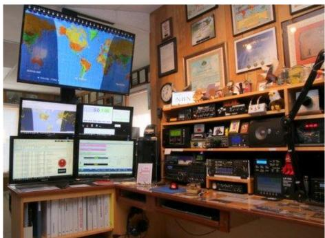
My station at home has a Yaesu FTdx5000, an Elecraft K2, and hopefully soon a K4. For HF, I use a K4KIO Hex beam antenna, a GAP Challenger, and a SteppIR BigIR vertical primarily for 30, 40 and 75 meters. When required, I can add a bit of power with the Elecraft KPA 1500 amplifier. For VHF/UHF at home, I use my old reliable Yaesu FT 8800.
