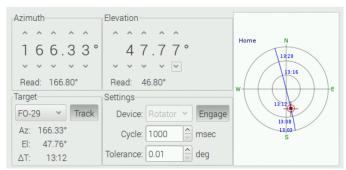
After further reading all the SARC documentation, I learned that if I used a Linux solution the limitation of the position not being reported back was eliminated. So I decided to use a Raspberry Pi 3B. Using this, I could build a Raspian computer for less than \$35 and also use the latest releases of the free gPredict (v2.2.1 at the time) software to control my rotator, and having Auto Track.
