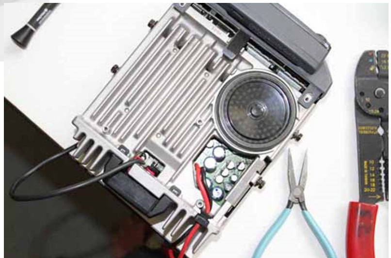
Power cable exit with strain relief
