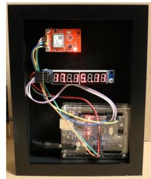
The photos are of me holding the bare unit, and then the finished project in a nice shadow box. The shadow box was on sale at Michael's Arts and Crafts store (\$4.50). Looking at the completed project, the antenna is the small board, the *Arduino* UNO is the large
